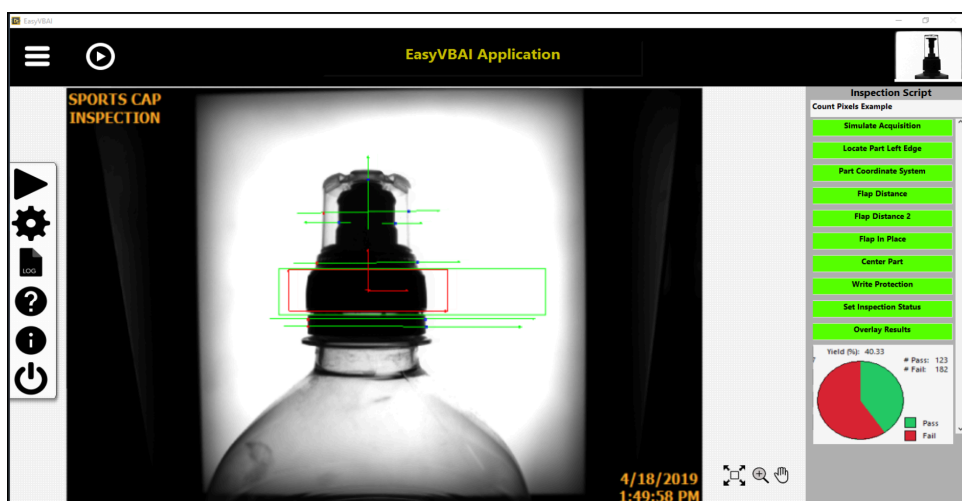
Automatic Sports Cap Inspection System display at an expo by Noreside Engineering Noreside built the conveyor/transport system, auger and reject station. Link to the setup video
